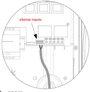
Connect the eSense cables using the opposite diagram
