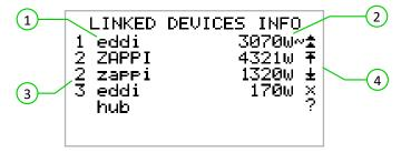
This screen lists all the linked devices (1) and the priority setting for each device (3) The current device is shown in CAPITAL letters. To the right of each device is the real-time output power level (2) The right side of the screen has symbols to show the status of each device (4) Refer to the table on the next page for the meaning of each symbol.
