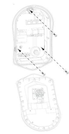
Using the fixing kit provided secure unit to the wall ensuring the grommets are used to maintain its IP integrity (Note: if using the rear cable entry remember to insert the mains cable before mounting to the wall!)
