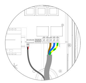
For single phase installations where 1 or 2 external / additional CT's are required, please follow the above diagram to connect the CT's using the extra 2 CT terminals in the same way if required. Positive (+) = Red Negative (-) Black
