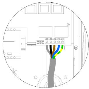
For 3 phase installations without the need for hardwiring an external CT please use the above diagram.
