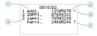
All linked devices (1) are listed in the DEVICES screen, the device shown in CAPITAL letters is the device currently being viewed. The serial number of each device is shown on the right (2)
